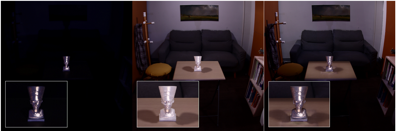
Fig. 12: Visually altering the surface material of the diffuse statue to a mirror-like specular appearance in three lighting conditions: (left) in a dark room, (center) under typical room lighting, and (right) under the proposed projector-based environmental lighting.
