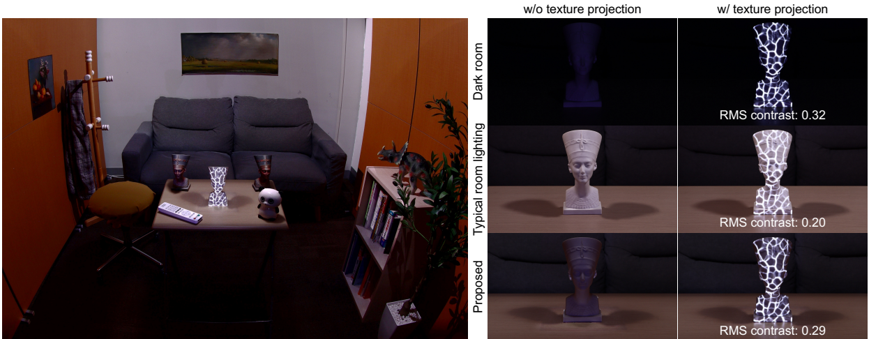
Fig. 1: The proposed projection mapping system mitigates the reduction in contrast under environmental lighting. The left image provides an overall view of the texture projection in a well-lit room using the proposed technique. The crack pattern texture is projected onto the white statue located at the center of the desk. The images on the right show enlarged views of the statue without (left) and with (right) the texture projection. These images were captured in three different lighting conditions: a dark room, where projection mapping is typically conducted; under typical room lighting with LED lights; and under the proposed environmental lighting using projectors. The results demonstrate that our technique reproduces typical room lighting using multiple projectors and enhances the contrast of the projected result on the target surface.
