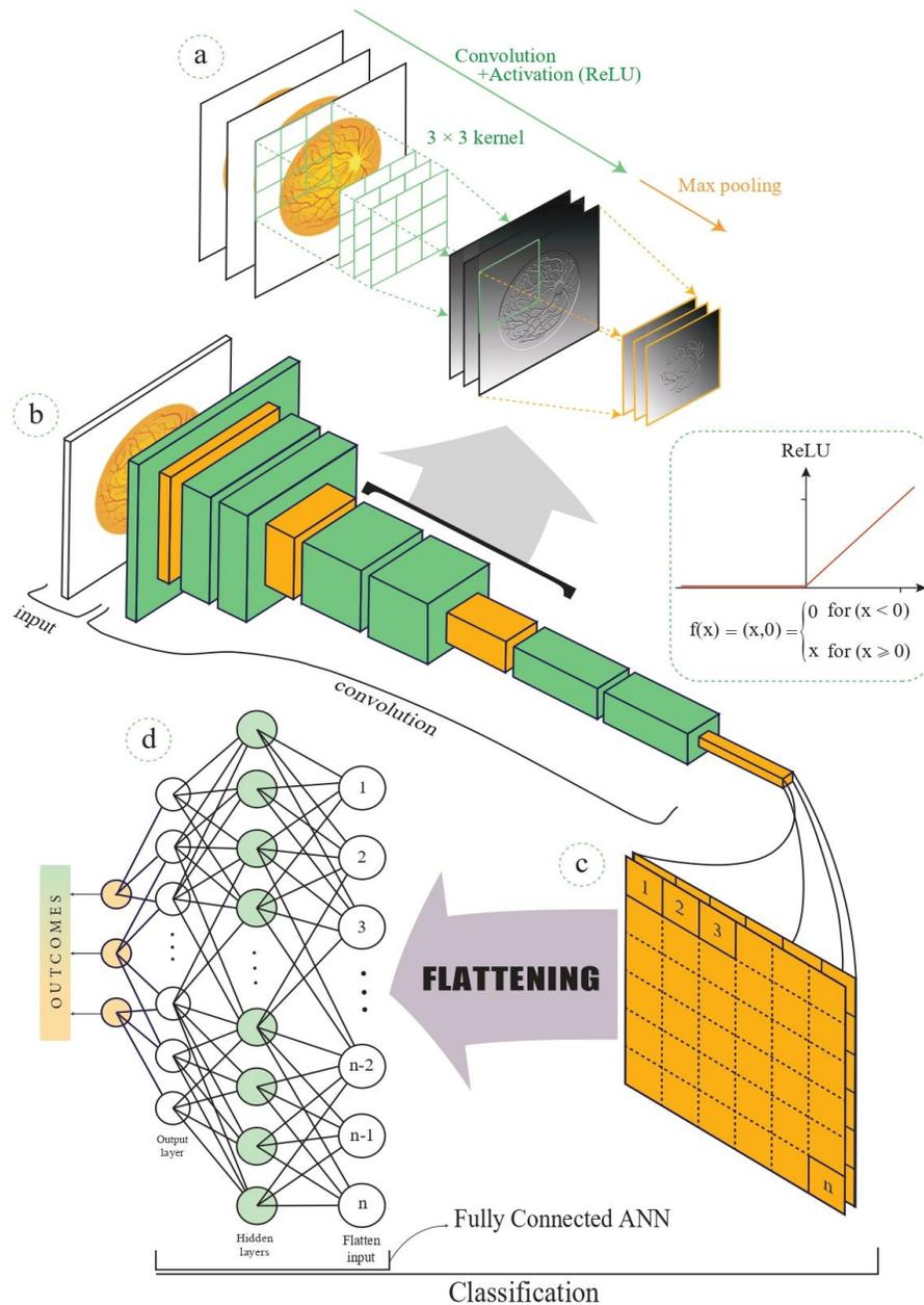
**Figure 5.** A detailed look at the architecture of a convolutional neural network (CNN) for image analysis. a: The convolutional layers (green) use kernels that slide over the three-channel RGB image to recognize key features from
