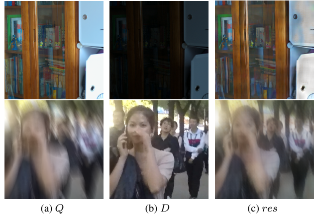
Figure 4. Result of frequency components mixing. An encoder ( \Phi ) extracts features from Q and D . We mix the frequency components using the amplitude of \Phi(Q) and the phase of \Phi(D) . Then the feature with mixed-frequency component is decoded into the pixel domain.
