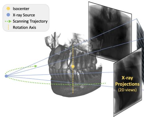
**Fig. 7.** Overview of Sparse-view Neural Attenuation Fields (SNAF) [18]. An X-ray source systematically traverses around the region of interest, producing sparse projections captured by a flat-panel detector positioned on the opposite side.
