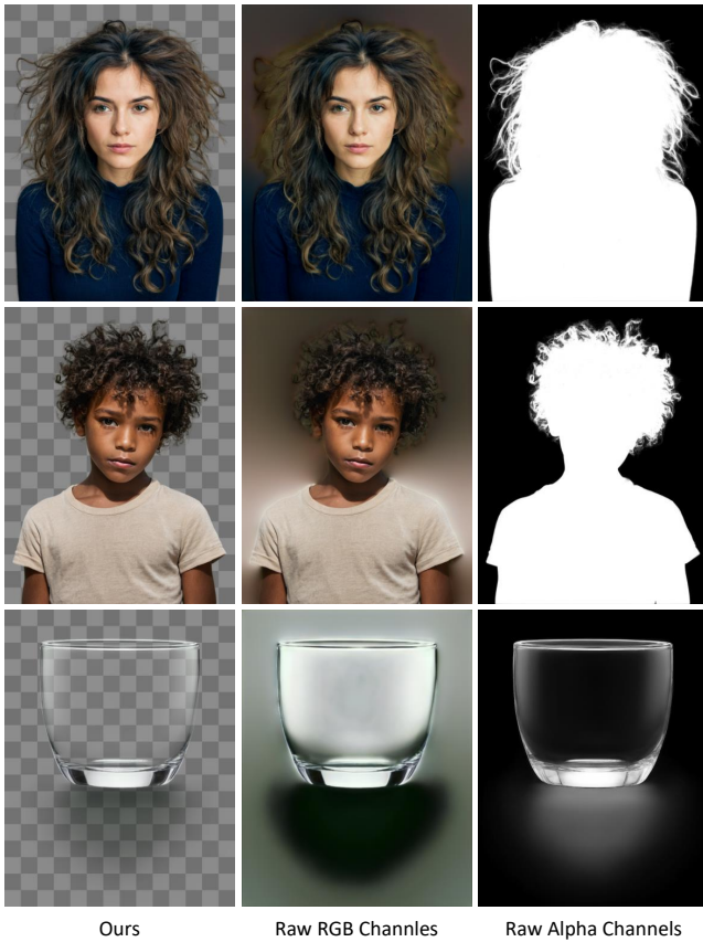
Fig. 14. Raw outputs of the RGB channels and alpha channel. We present the raw RGB and alpha channel for evaluation. The prompts are “woman with messy hair”, “boy with messy hair”, and “glass cup”.
