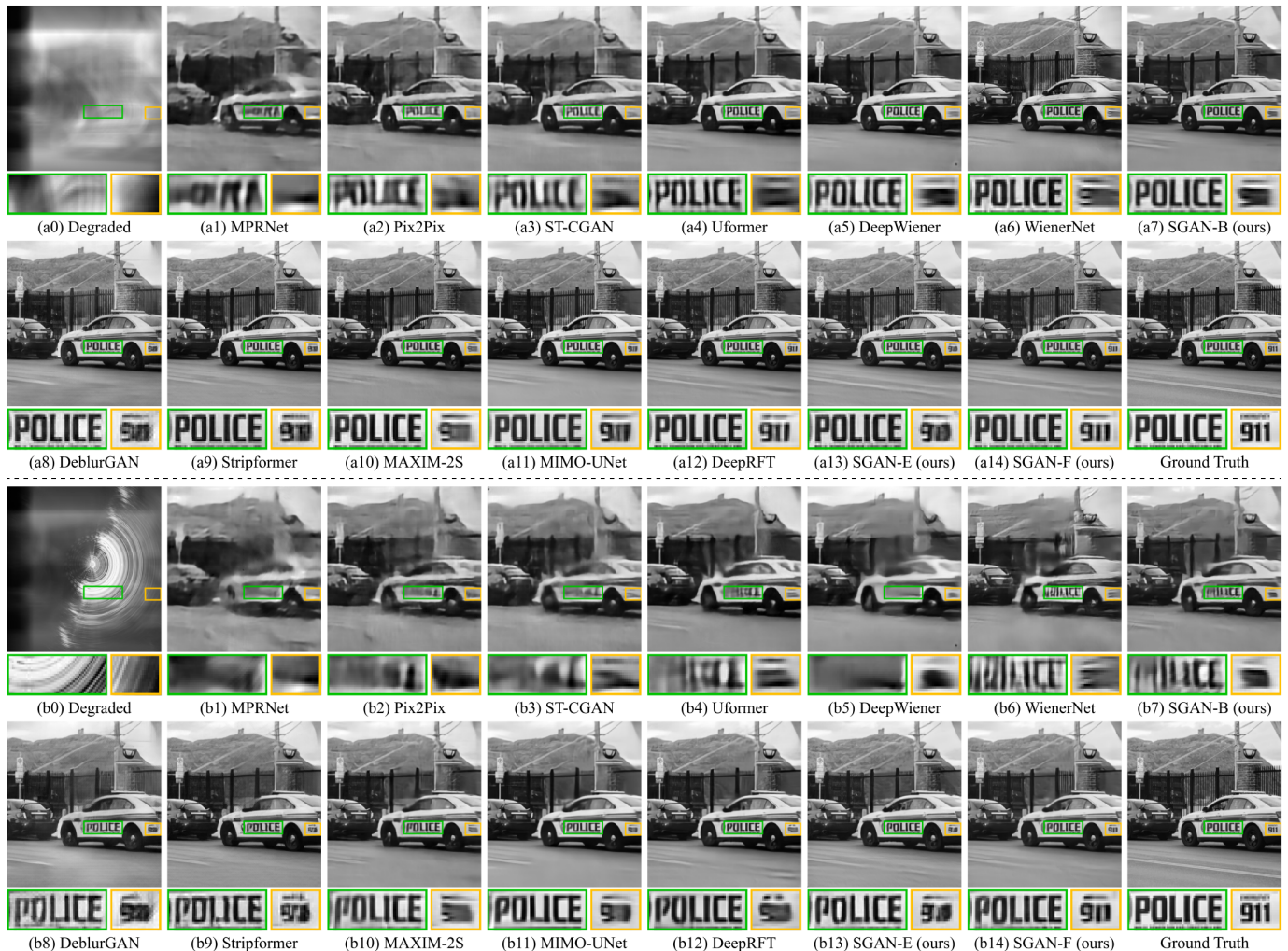
Fig. 5: Evaluation of laser-dazzle protection in simulation. Our SGAN-B/E/F models are compared with alternative methods for image restoration of a laser-free case ( \alpha_l = 0 ) in rows 1 and 2, and a damaging laser-dazzle case ( \alpha_l = 1e6 ) in rows 3 and 4. In each case, images restored by low- and high-performing models are respectively shown in the top and the bottom strips. MPRNet [129], Pix2Pix [146], and ST-CGAN [172] yield significantly distorted results in both cases. Uformer [111], DeepWiener [92], WienerNet [91], and our SGAN-B deliver reasonable recoveries, but perform poorly in the presence of laser dazzle. DeblurGAN [152], Stripformer [126], and MAXIM-2S [118] show improvements against laser dazzle in terms of coarse image features; however, fine image details (see the zoom-in image patches outlined by yellow boxes) remain unrecognizable regardless of the laser strengths. Without a laser, high-frequency features become recognizable in the images restored by MIMO-UNet [125], DeepRFT [127], and our SGAN-E. Among all, our SGAN-F produces the consistently highest fidelity image in both the laser-free and laser-dazzle cases.
