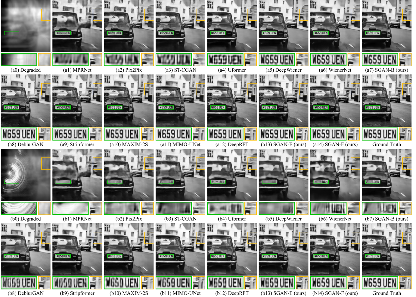
Fig. 3: Evaluation of laser-dazzle protection in simulation. Our SGAN-B/E/F models are compared with alternative methods for image restoration of a laser-free case ( \alpha_l = 0 ) in rows 1 and 2, and a damaging laser-dazzle case ( \alpha_l = 1e6 ) in rows 3 and 4. In each case, images restored by low- and high-performing models are respectively shown in the top and the bottom strips. MPRNet [10], Pix2Pix [11], and ST-CGAN [12] yield significantly distorted results in both cases. Uformer [14], DeepWiener [5], WienerNet [13], and our SGAN-B deliver reasonable recoveries, but perform poorly in the presence of laser dazzle. DeblurGAN [15], Stripformer [17], and MAXIM-2S [18] show improvements against laser dazzle in terms of coarse image features; however, fine image details (see the zoom-in image patches outlined by yellow boxes) remain unrecognizable regardless of the laser strengths. Without a laser, high-frequency features become recognizable in the images restored by MIMO-UNet [16], DeepRFT [7], and our SGAN-E. Among all, our SGAN-F produces the consistently highest fidelity image in both the laser-free and laser-dazzle cases.
