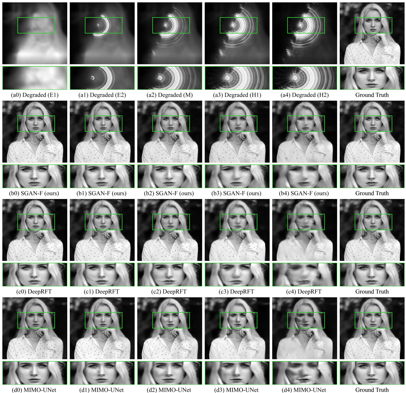
Fig. 4: Evaluation of the the robustness of laser dazzle protection against five degradation stages: easiest (E1), easy (E2), medium (M), hard (H1) and hardest (H2) from columns 1-5. Compared to the ground truth image shown in column 6, the imaging conditions deteriorate as laser dazzle and photon noise increase, and the strength of background illumination decrease. A set of phase-coded images (row 1) illustrates the progressive worsening of image quality through these stages. The image restoration performance of our SGAN-F (row 2) is compared with that of DeepRFT (row 3) and MIMO-UNet (row 4). Although all models produce high-quality recoveries of the laser-free scene, DeepRFT and MIMO-UNet showcase a significant increase in distortion from E1 to H2. In contrast, our SGAN-F model consistently delivers higher fidelity restorations at every stage, demonstrating its superior robustness against the challenging imaging condition.
