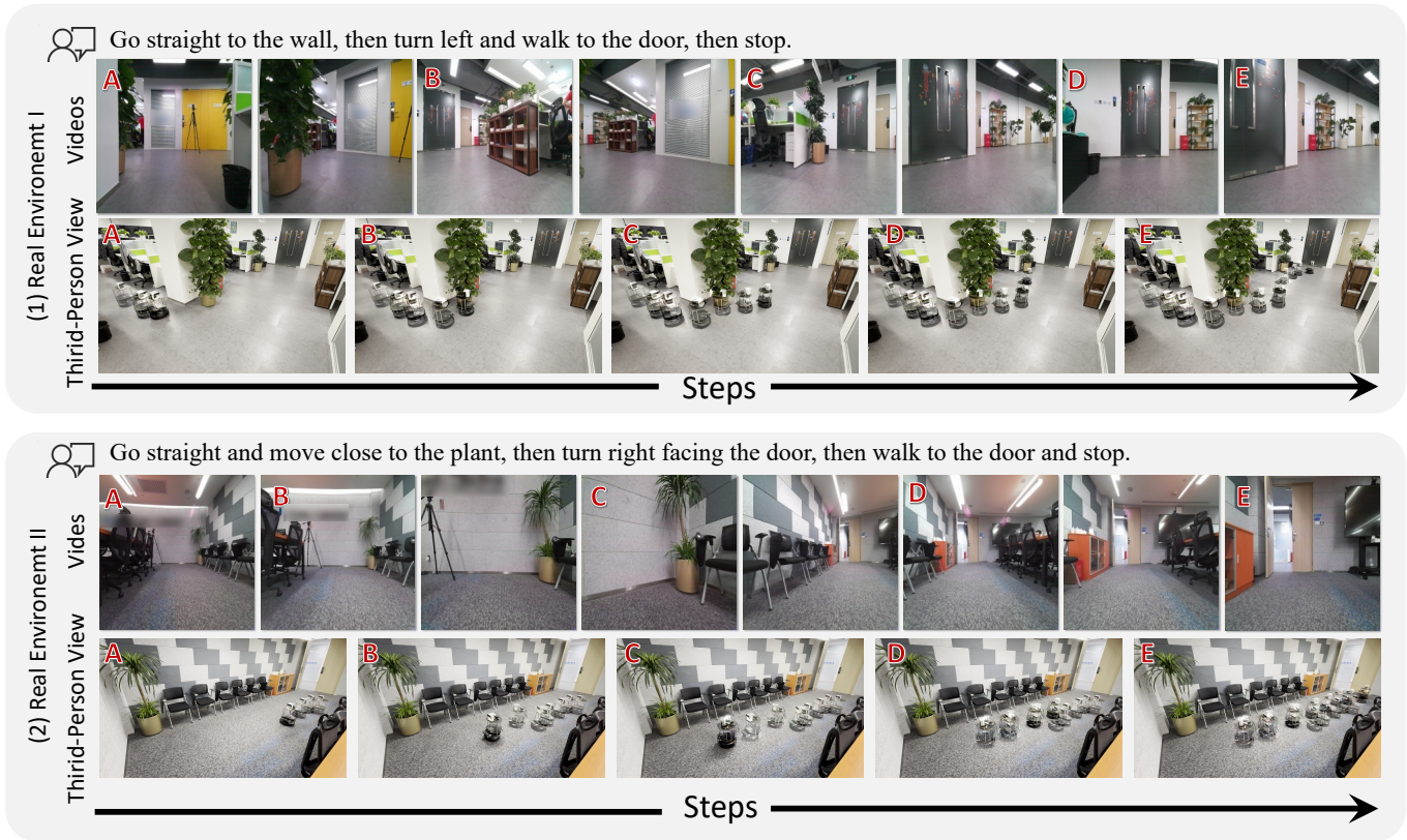
Fig. 7: Visual results of our method in a real-world environment. In each real environment example, from top to bottom are instruction, robot perspective video, and third-person view video.
