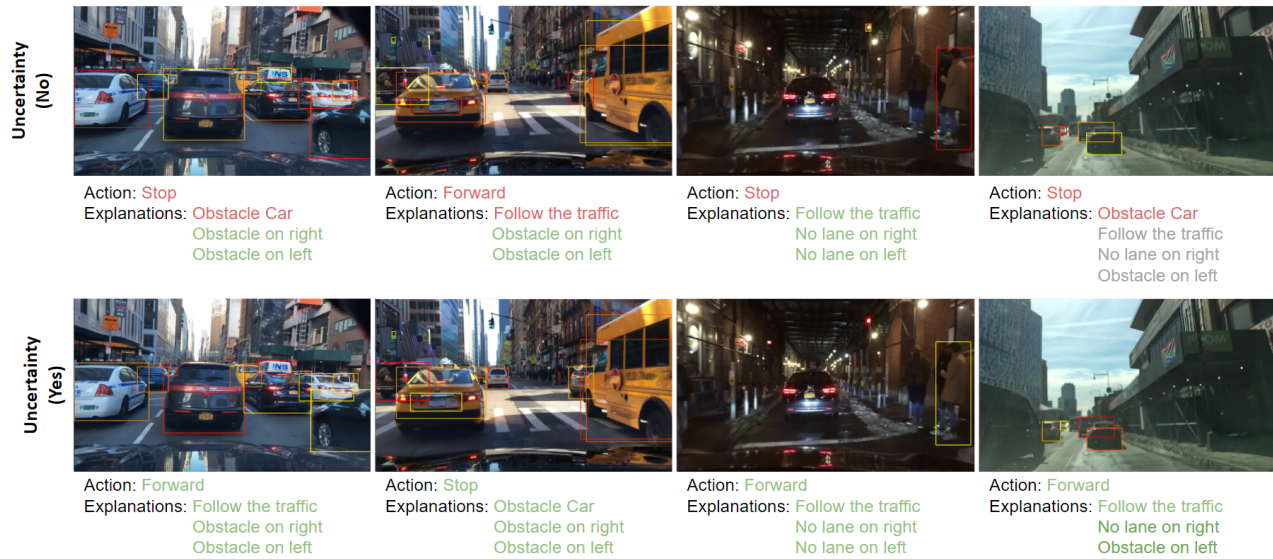
Figure 2: Comparison with Original OIA: the color of bounding boxes reflects the rank of importance (red to yellow = most to least important), and the color of actions and explanations reflects the correctness (green=correct, red=incorrect, gray=missing)
