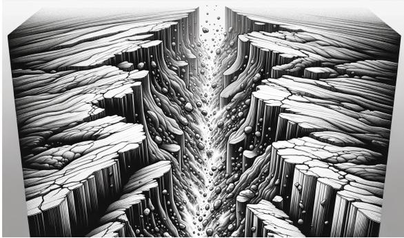
FIG. 1 Artistic representation of the magnified rough interface between two plates in sliding contact, where asperities grinding give rise to debris particle formation.
