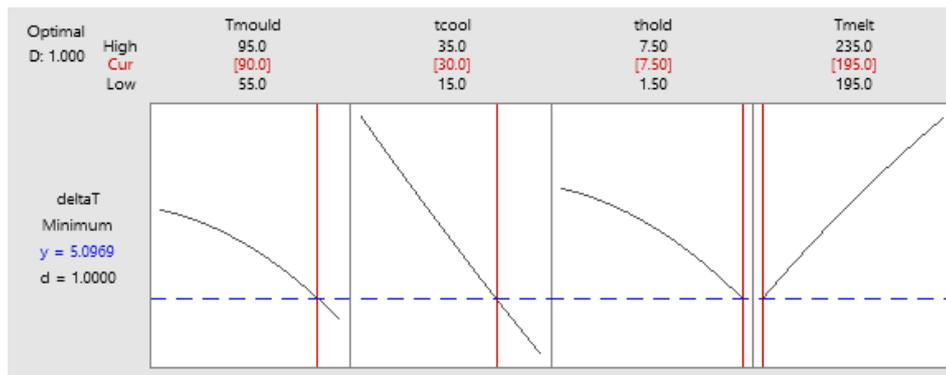
Fig. 10. Optimisation by desirability function for single response  $\Delta T$
