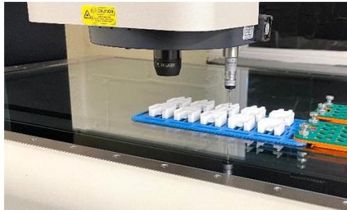
Fig. 7. OGP Smartscope CNC 500 measuring the main dimensions of Clip.
