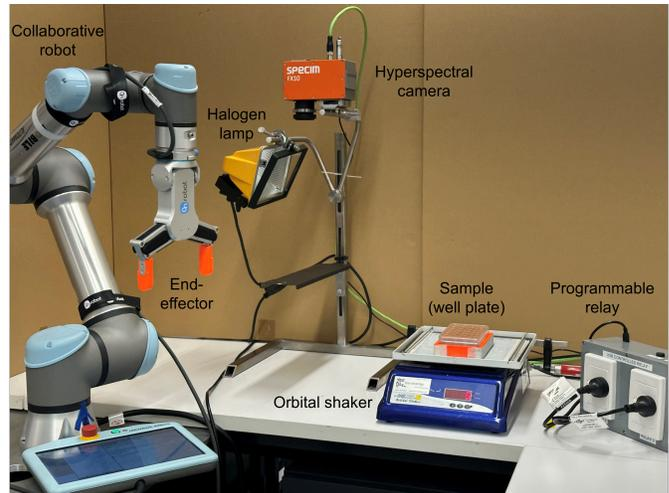
Fig. 1: Robot-aided hyperspectral mapping and data sampling.
