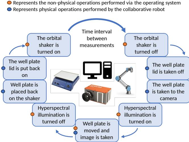
Fig. 5: Schematic diagram of the imaging procedure. The lid manipulations are crucial steps to minimise evaporation when idle and mitigate any potential artefacts during the imaging process.
