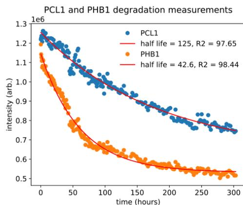
Fig. 8: The degradation of PCL1 and PHB1 were measured over the course of two weeks. PBS of strength pH 14 was used to attain these results.
