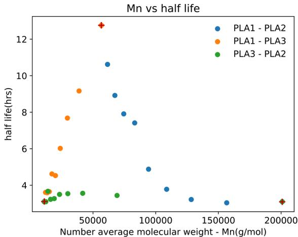
Fig. 11: Blend of pairs of polymers demonstrating the effect of molecular weight and end groups. The “+” on a data point represents that it’s a shared point between two blends.
