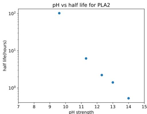
Fig. 9: Illustrates the effect of pH strength on the half-life of PLA2
