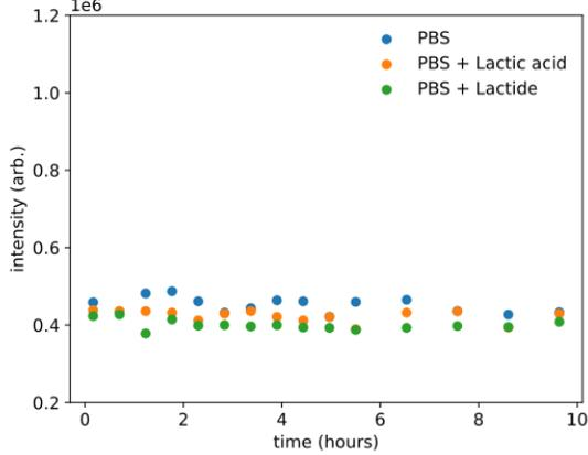
Fig. 4: Total light reflected by the control samples. Lactide and Lactic acid aren't contributing to a signal change (plotted with the same range as the actual results shown in subsequent figures). The standard deviation of reflection intensity values for these controlled samples is less than 5% of their average values for all cases.
