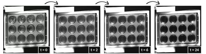
Fig. 3: A black and white representation of hyperspectral images, used to measure the degradation rate of polymers. The degradation process is evident as time (in hours) progresses from the left to the right image.
