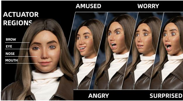
Figure 3. Virtual Performer Sophia and Her Facial Expression Samples. The brow region features 5 motors allowing for eyebrow lifting, while the eye and eyelid area is equipped with 11 actuators for blinking and eye movement. Additionally, the nose region contains 2 motors, and the mouth area includes 14 motors that control movements of the mouth, tongue, jaw, and surrounding muscles, enabling a wide range of expressive capabilities.
