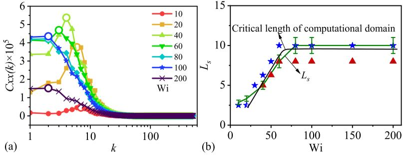
Figure 3: (a) Spectra of the streamwise elastic energy  $C_{xx}$  at  $y^* \approx 0.5$  at different  $Wi$ ; (b) Characteristic scales  $L_s$  of the  $C_{xx}$  and the critical computational domain at different  $Wi$ , where  $L_s = 20/k_p$  and  $k_p$  is the peak wavenumber obtained from  $C_{xx}(k)$ .
