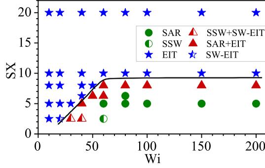
Figure 2: Phase diagram of flow states at different  $Wi$  obtained by different computational domain. SSW: steady sheets near the wall; SW-EIT: EIT occurrence near single wall; ”+”: the alternative occurrence of different states.
