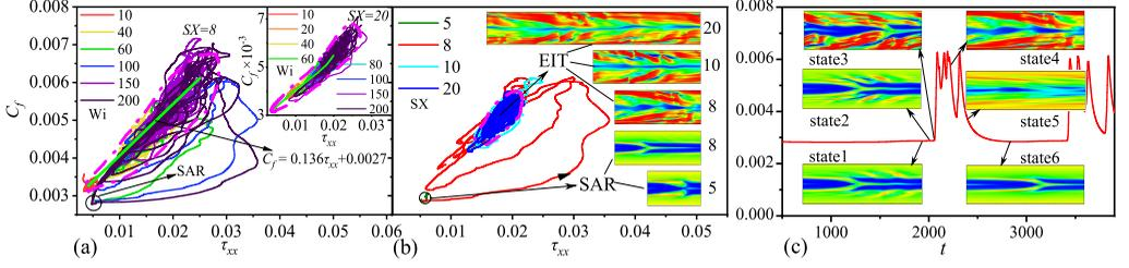
Figure 4: Dynamical and structural evolution cycles of (a)  $C_f$  with  $\tau_{xx}$  for different  $Wi$  at  $SX = 8$  and  $SX = 20$ ; (b)  $C_f$  with  $\tau_{xx}$  for different  $SX$  at  $Wi = 100$  (inset figures present the snapshots of streamwise extension fields  $C_{xx}$  obtained by different  $SX$  corresponding to the typical state); (c) structure intermittency at  $Wi = 100$  and  $SX = 8$ .
