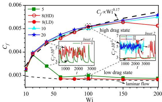
Figure 1: Statistical  $C_f$  of viscoelastic fluid flow at different  $Wi$  obtained by different computational domain. Two insets are the instantaneous  $C_f$  at two typical  $Wi$  of 40 and 100, respectively. Note: The red open and closed circle symbols represent the average  $C_f$  for different stable stages at  $SX = 8$  under the same  $Wi$ . The dashed line corresponds to  $C_f$  in laminar regime of FENE-P fluid at different  $Wi$ .
