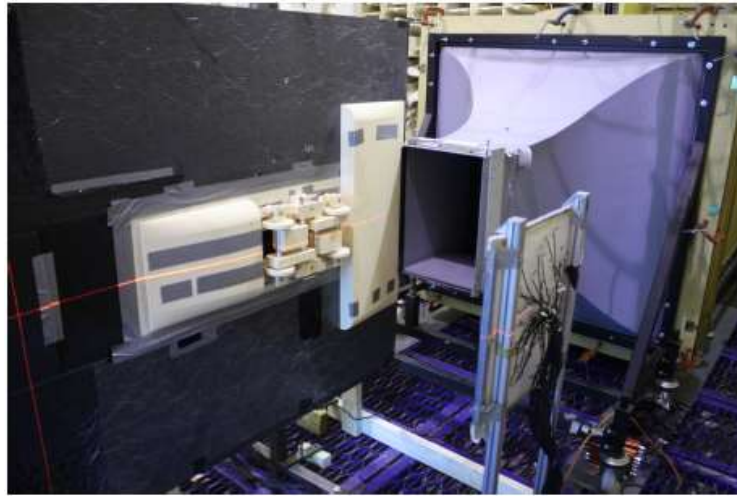
Fig. 13. Experimental set-up showing the 1:10 scale simplified bogie inside a simplified bogie cavity.
