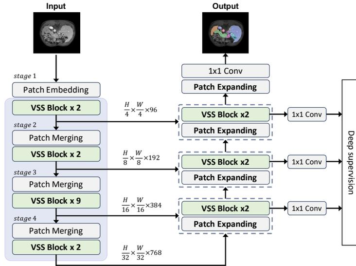
Fig. 2. The overall architecture of Swin-UMamba<sup>†</sup>.
