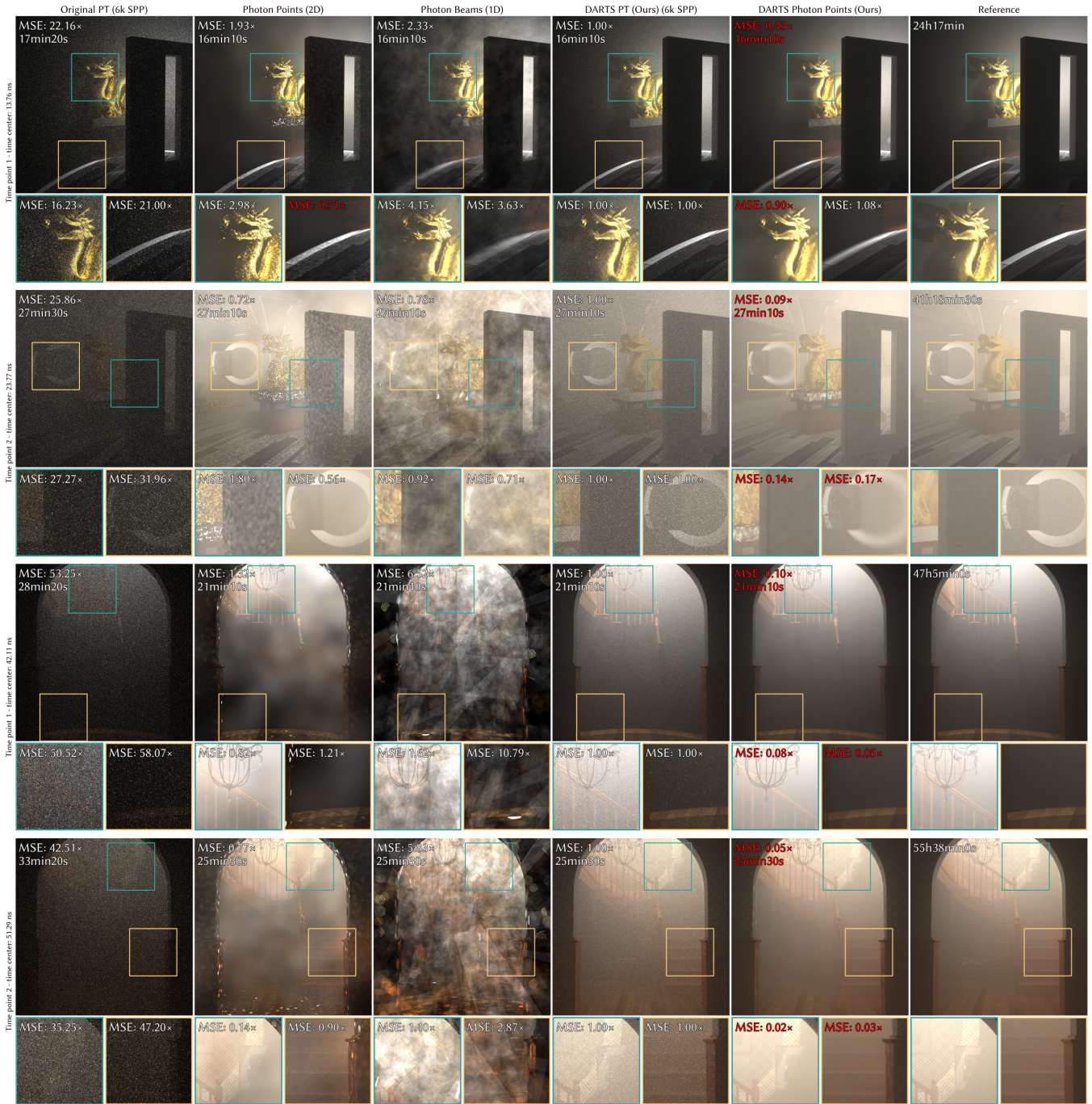
Fig. 7: Time-gated rendering experiments. For each scene, we present the time-gated images rendered by five different methods (organized by column) in two different time intervals (shorter and longer target path lengths). Each image will have two selected areas displayed in magnified views. For original and the proposed methods, we use 6k SPP to render each image and the photon based methods have rendering time equal to the proposed method. We set the MSE of our DARTS PT to be 1, and MSE relative ratios and rendering time are displayed on the top right of each image. The best statistics (row-wise) are highlighted in red . The leftmost texts describe the time point and the corresponding interval center of the rendered images. The original outputs are in HDR format, we therefore normalize the images with their 0.99 quantiles and clamp the output to [0, 1] . It can be seen that our DARTS PT (4th column) and DARTS photon points (5th column) methods have greatly improved rendering quality, compared to their original counterparts. Notably, photon points equipped with DARTS can achieve noise-free rendering with no obvious visual artifacts.
