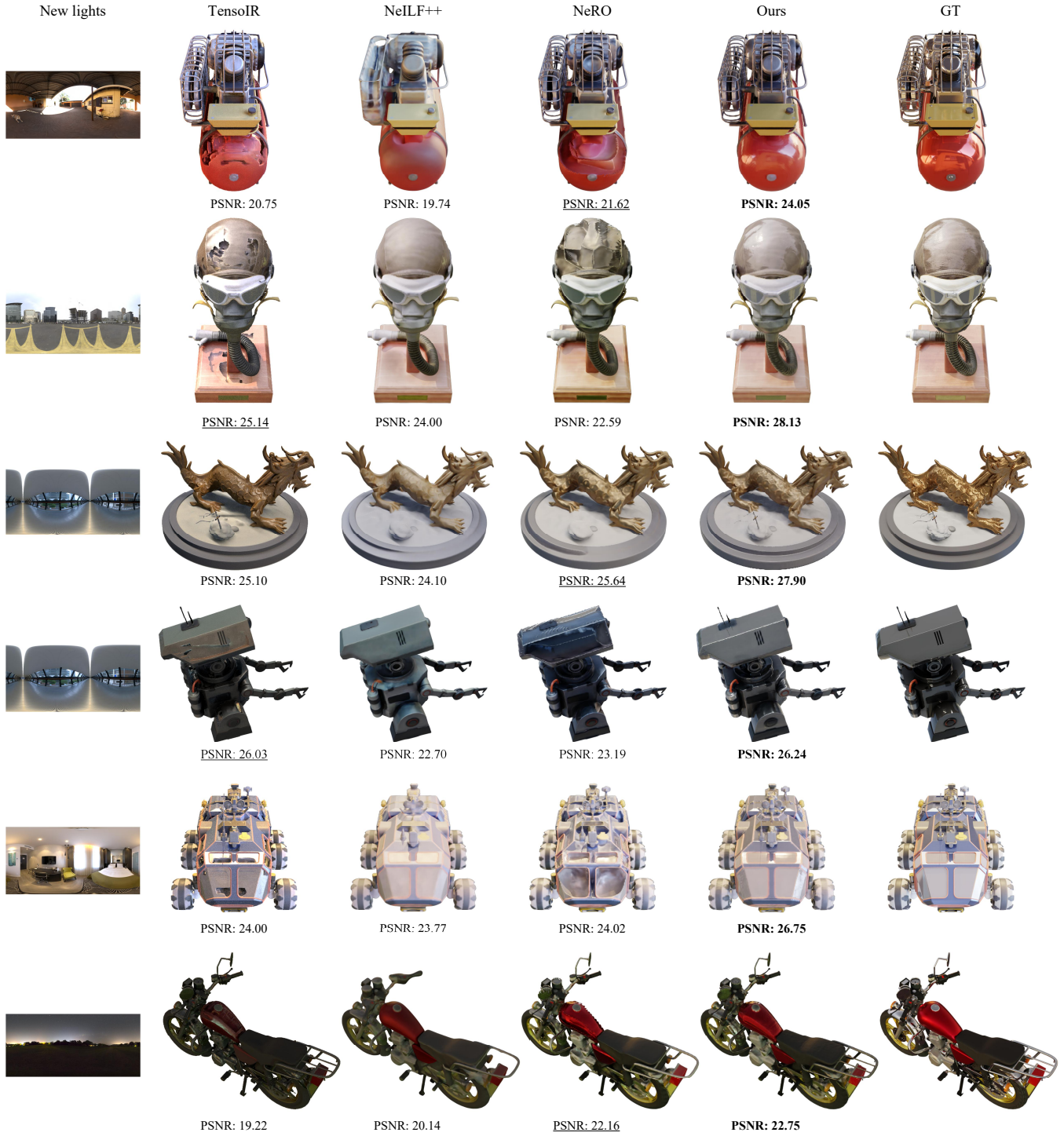
Fig. 3. Comparison of relighting results among our method, TensoIR [Jin et al. 2023], NeLF++ [Zhang et al. 2023] and NeRO [Liu et al. 2023] on our synthetic dataset.
