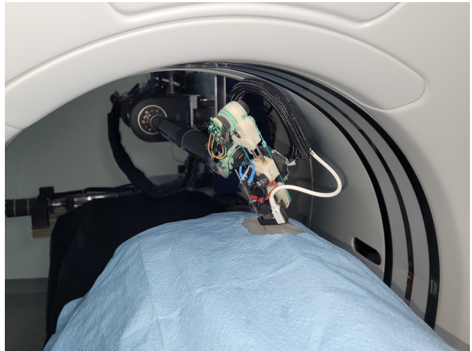
Fig. 1: Needle insertion within imaging bores provides direct volumetric visualization of the anatomy and tool, improving the accuracy of needle insertion procedures such as retroperitoneal biopsy and lumbosacral spine nerve block. However, this enclosed environment limits the space for manipulation and line-of-site visibility for devices. CRANE overcomes these challenges with its cable-driven serial link design and integrated planning-control method to enable fully in-bore dexterous needle manipulation without requiring manual setup.
