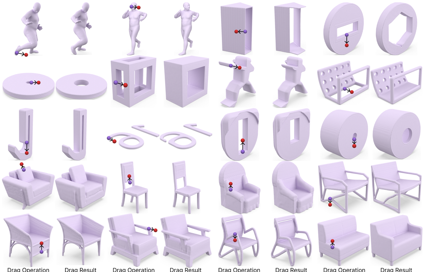
Fig. 11. Visual results for the drag operator. By providing a pair of source point (in purple) and target point (in red), our method is capable of modifying a diverse range of shapes to produce high-fidelity results that match the drag operations.
