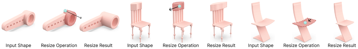
Fig. 8. Visual results of the resize operator. Our method enables one to select a region (in red) and resize it along a certain axis (black arrow) about a chosen anchor point (blue dot). The edited results are produced by matching the resize operations.
