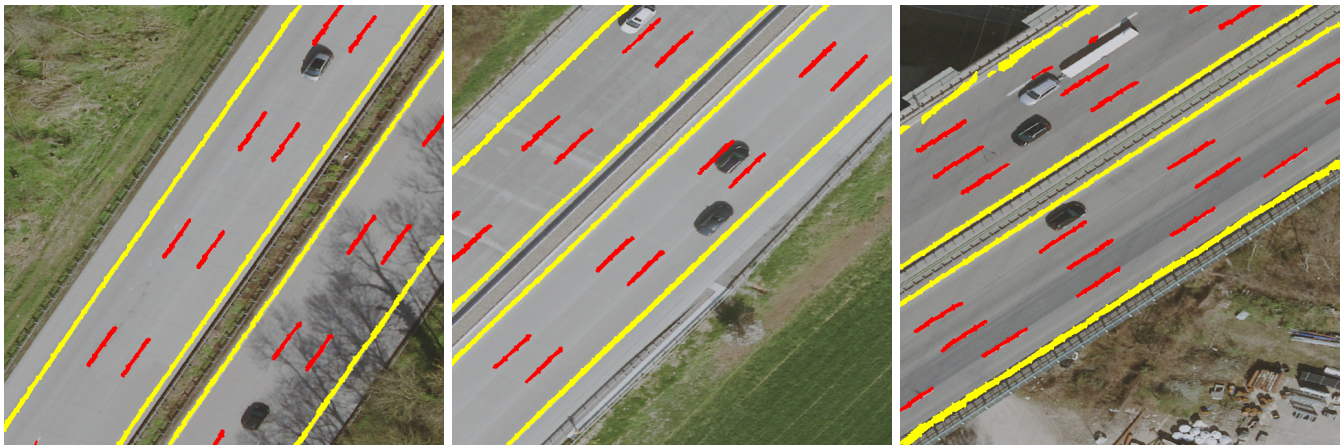
Fig. 6: Predictions on the KAI test dataset published in [29]. Line segment classification is used here to distinguish heterogeneous objects. All variants also estimate a direction of the marking and thus correctly describe the direction of travel of the lane. Image source of aerial photos: ©City of Karlsruhe — Liegenschaftsamt
