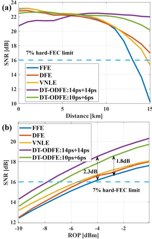
Fig. 8. Performance of the DT-ODFE in (a) varied fiber distance and a fixed ROP of -6dBm, and (b) varied ROP at a fixed 10km distance.
