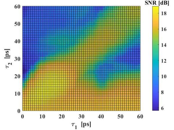
Fig. 5. 2D-optimization results of the delays of the DT-ODFE with a  $10\text{km}$  distance and  $50\text{Gbaud}$  signal.
