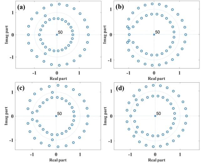
Fig. 3. System pole-zero plots of different distances and optical coefficients of (a)10km, w/o DT-ODFE, (b)10km,  $\tau_1$ : 14ps;  $\tau_2$ : 14ps, (c)15km, w/o DT-ODFE, and (d)15km,  $\tau_1$ : 14ps;  $\tau_2$ : 14ps.
