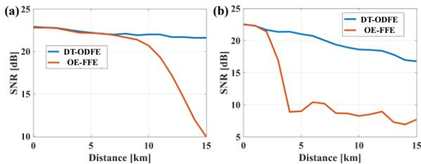
Fig. 7. Performance comparison between DT-ODFE and OE-FFE of (a)50 Gbaud and (b)100 Gbaud.
