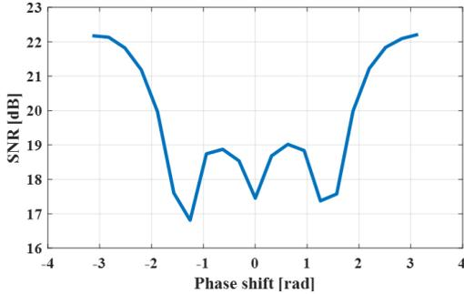
Fig. 6. SNR versus phase shift with  $10\text{km}$  distance,  $14\text{ps}$   $\tau_1$  and  $14\text{ps}$   $\tau_2$ .
