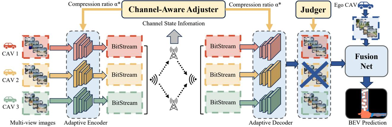
Fig. 2: Overall architecture of SmartCooper consists of three stages. (1) Network optimization: determining the parameters of CSI to output the optimized compression ratio  $\alpha^*$ . (2) Transmission & Judgement: Each CAV transmits its compressed image data to the Ego CAV and receives a judgment. (3) Fusion: the qualified reconstructed images are combined with the Ego CAV’s image to generate a BEV through the fusion net.
