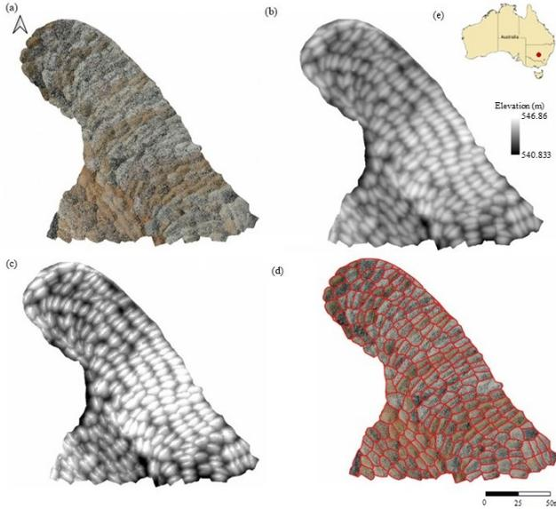
**Fig. 2.** (a) Orthomosaic and (b) digital surface model (DSM) and (c) hillshade representation of selected area of spoil piles, (d) ground truth segments and (e) location of selected area.
