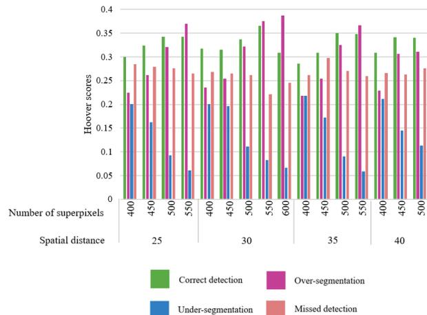
**Fig. 4.** Hoover metrics scores for specific parameters in Simple Linear Iterative Clustering (SLIC). The correct detection score is maximised at spatial distances of 30 and 550 superpixels. However, at these parameter settings, the oversegmentation score surpasses the correct detection score. Increasing the number of superpixels while maintaining a spatial distance of 30 leads to a rise in oversegmentation, accompanied by a decline in correct detection.
