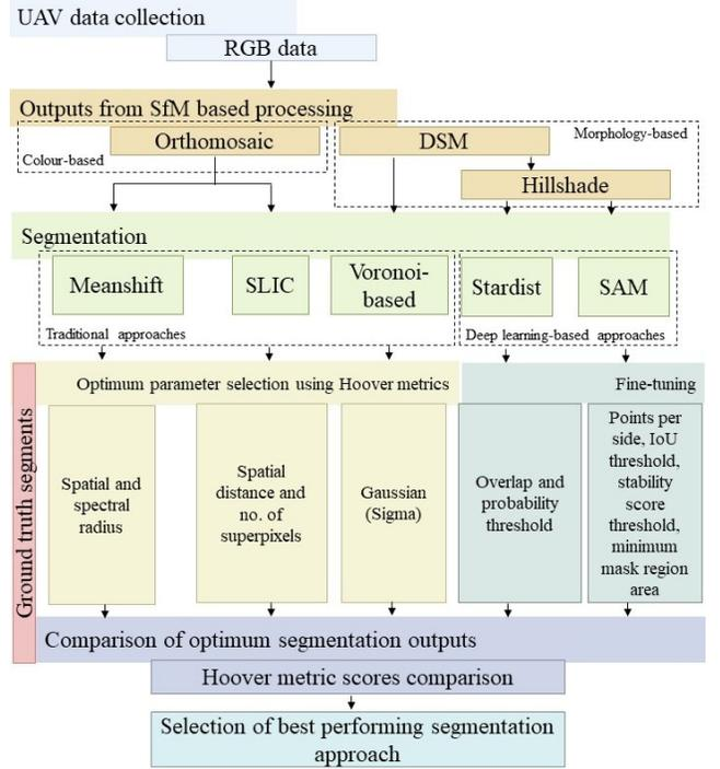
**Fig. 1.** Workflow employed for the comparative analysis of traditional and deep learning-based segmentation approaches in the context of coal spoil pile segmentation.
