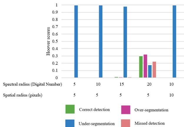
**Fig. 3.** Hoover metric scores corresponding to parameters in mean shift segmentation. Optimal performance, indicative of accurate detection, is attained with a spectral radius of 20 digital numbers and a spatial radius of 5 pixels. Alternative parameter combinations yielded increased level of under-segmentation.
