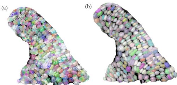
**Fig. 6. (a)** Star-convex polygons parameterised by the radial distances in hillshade representation of spoil pile and **(b)** StarDist segmentation results.
