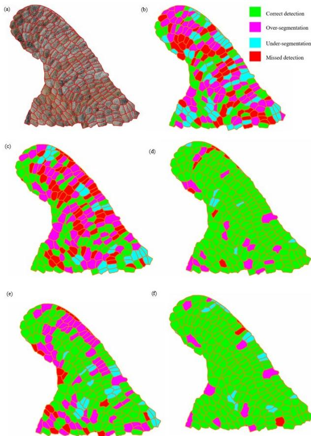
**Fig. 10.** (a) Ground truth segments and Hoover scores on ground truth for (b) mean shift algorithm, (c) simple linear iterative clustering and (d) Voronoi-based segmentation, (e) StarDist segmentation and (f) segment anything model
