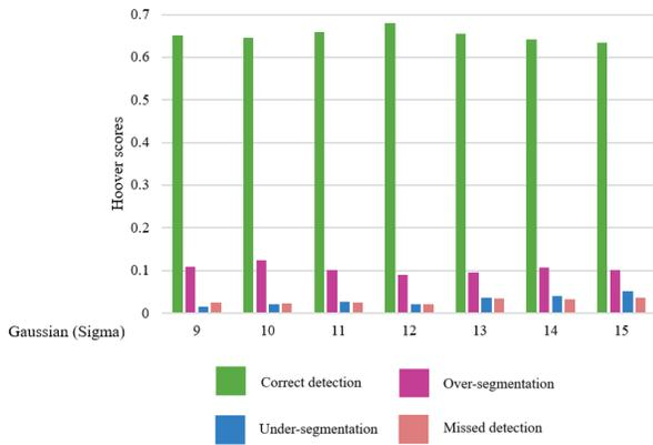
**Fig. 5.** Hoover metrics scores for corresponding parameters of Voronoi-based segmentation. The correct detection scores are presented in relation to the sigma values of Gaussian blurring. Notably, a superior correct detection score is observed at a sigma value of 12.
