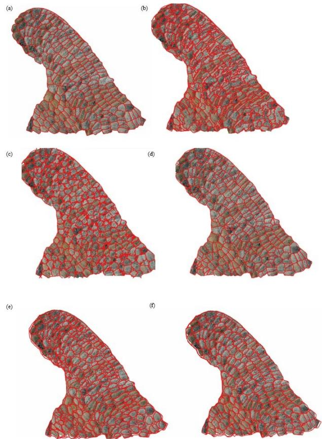
**Fig. 9.** (a) Ground truth segments and segmentation results of (b) mean shift algorithm, (c) simple linear iterative clustering, (d) Voronoi-based segmentation, (e) StarDist segmentation and (f) segment anything model
