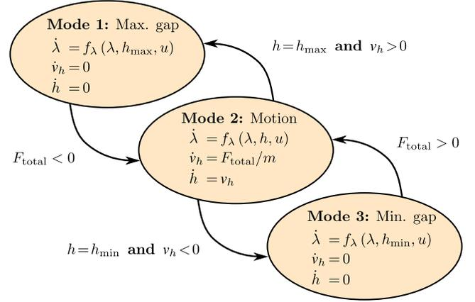
Fig. 2. Hybrid automaton to model the actuator dynamics. The motion of the plunger is restricted to  $h \in [h_{\text{min}}, h_{\text{max}}]$ . Variable  $v_h$  represents the velocity of the plunger along the gap direction.
