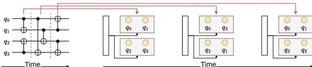
Fig. 1: Quantum circuit (timeslices in red) mapping into a modular architecture. The lower row shows how the mapping can be approached as a graph-partitioning problem.
