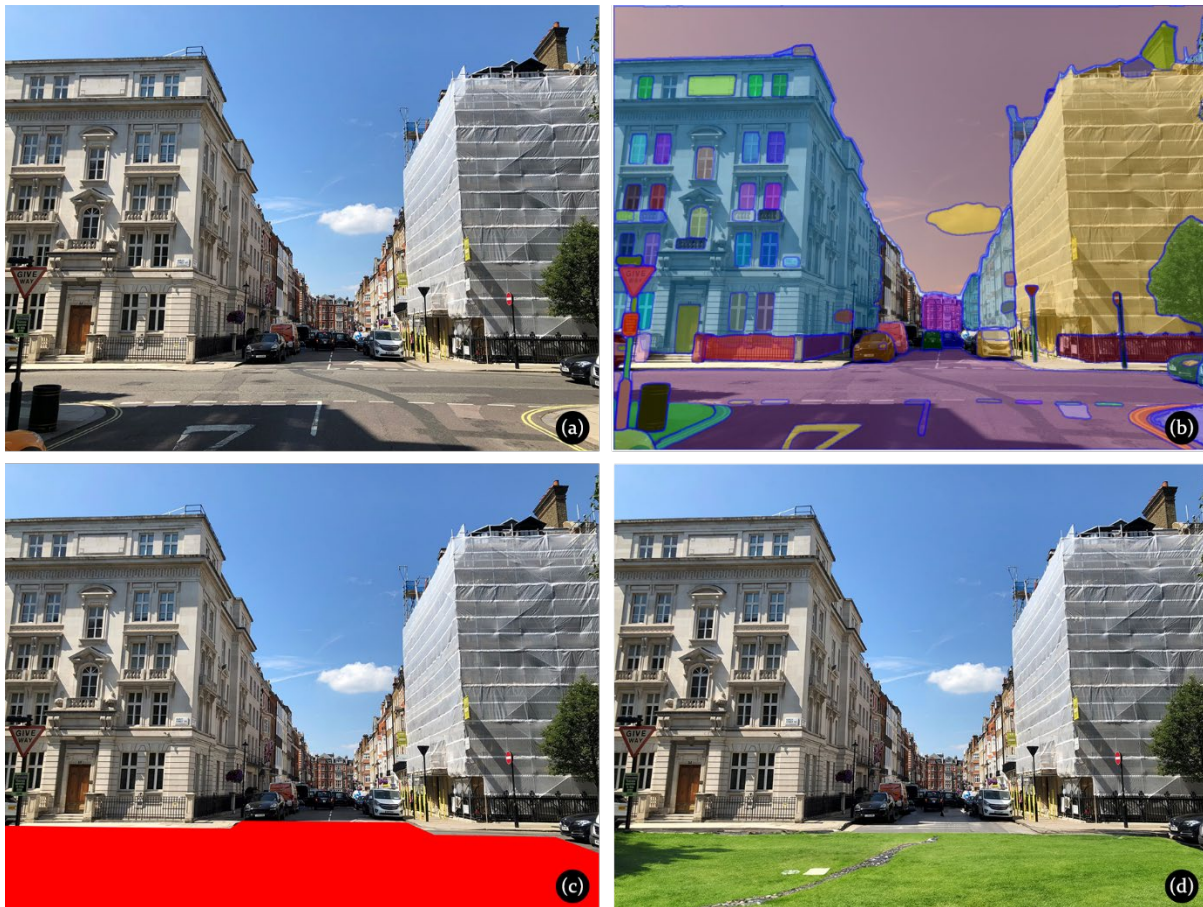
Figure 3: Sequential workflow demonstration in architectural design education: (a) original urban landscape input by a student; (b) automated segmentation via OneFormer highlighting distinct urban elements; (c) focused object selection and masking; (d) final SDXL-generated image reflecting textual design prompt integration.
