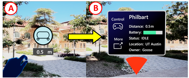
Fig. 2. [A] AR-label used to visualize agent type and location in the environment. Blue NATO symbol represents an unmanned ground vehicle (UGV). [B] AR-label, expanded with click, providing additional information and clickable “Control” and “More” buttons to access more control, command, and supervision functionalities.
