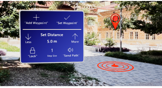
Fig. 3. Holographic waypoint options menu and red holographic marker presented to users to physically define a waypoint navigation goal for autonomous agents.
