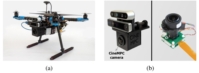
Figure 15. Experimental setup of hardware experiments. (a) CineMPC drone platform. (b) Left - Close view of the cameras. Top to bottom: RGB-D Camera, Odometry camera, and Cinematographic camera (inside the CineMPC box). Right - Close view of Cinematographic camera (outside the CineMPC box). Note the inclusion of motors designed to control zoom and focus in real-time.
