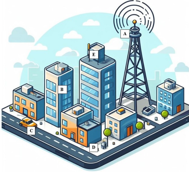
Fig. 2: A typical communication scenario with an adversarial actor. (A) represents the base station. (B), (C), and (D) are indoor, outdoor, and vehicular User Equipment (UE), respectively. (E) is an adversarial base station that has the capability to intercept, modify and re-transmit data coming from (A).
