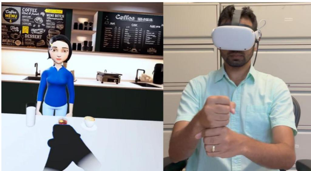
Figure 7. A side-by-side view of the system. The left and right sides show the VR and real-world views, respectively. The user is signing COFFEE, and the avatar is waiting to provide feedback.
