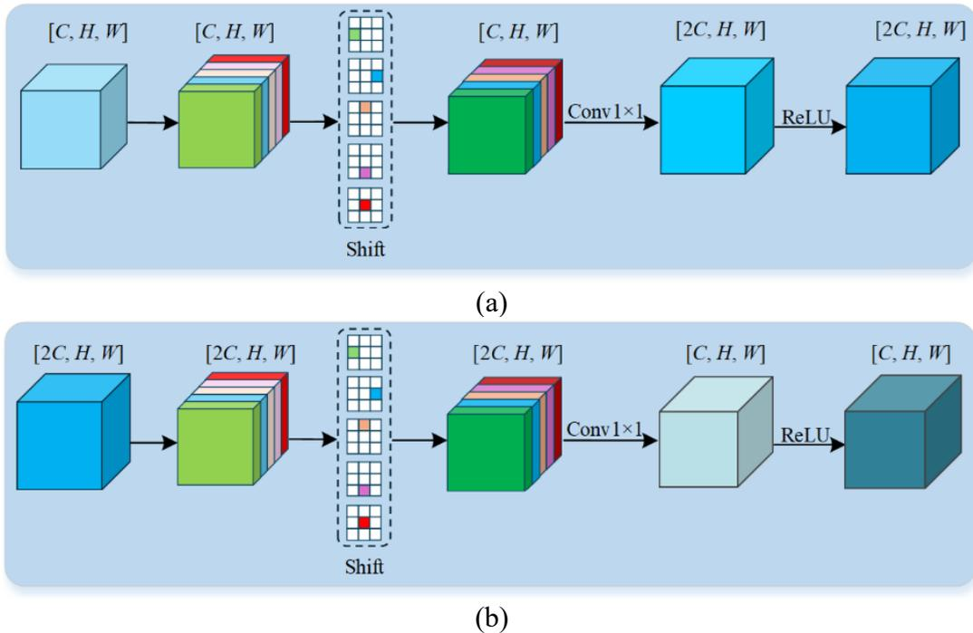
**Fig. 4** Shift convolution schematic. (a) Channel expansion shift convolution; (b) Channel compressed shift convolution.
