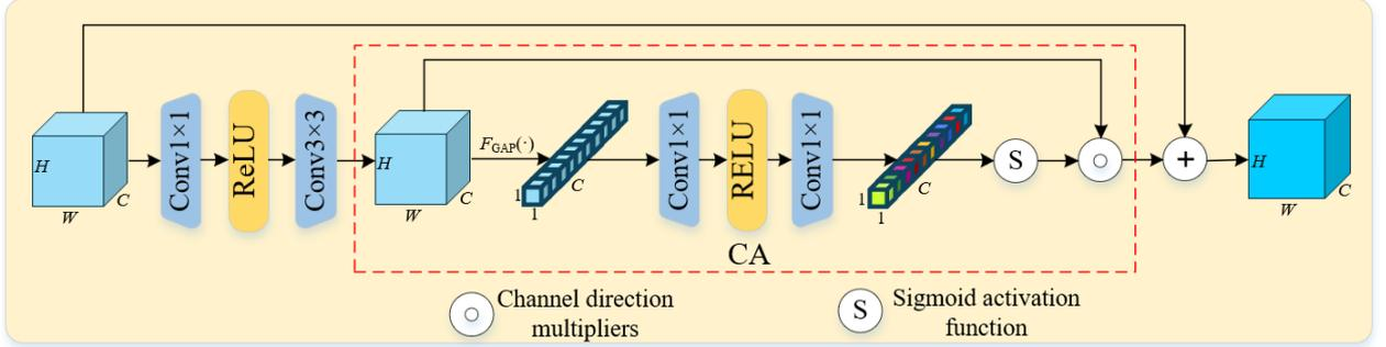
Fig. 8 Schematic of the low-parametric residual channel attention module.
