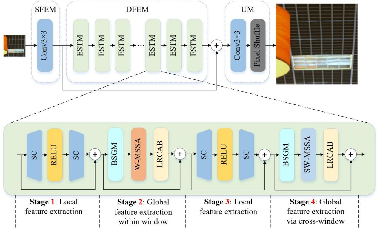
Fig. 3 Enhanced Swin Transformer image super-resolution reconstruction network
