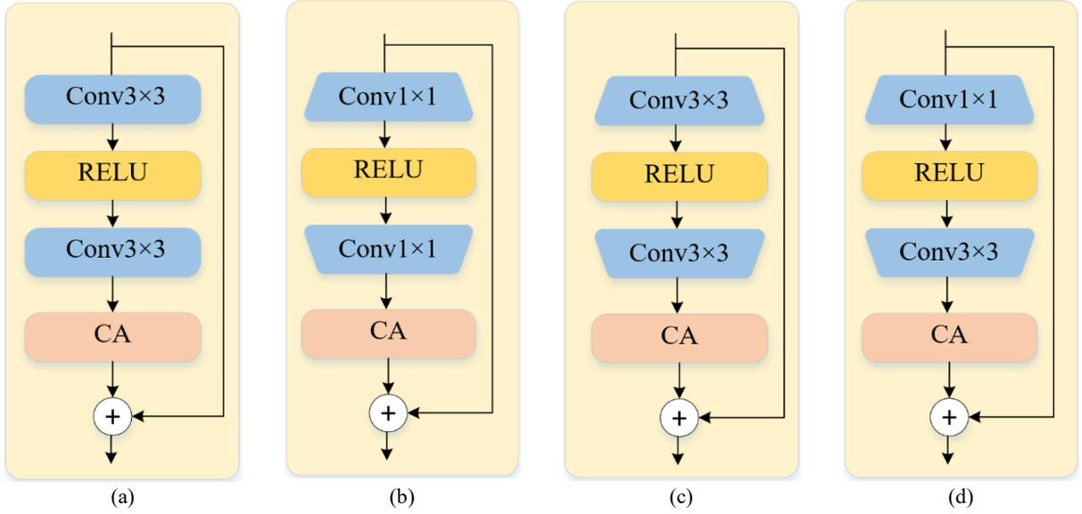
**Fig. 14** Comparison of low-parameter residual channel attention modules with other channel attention modules: (a) Original RCAB; (b) Two Conv1×1 RCAB; (c) Two Conv3×3 RCAB; (d) Conv1×1&Conv3×3 RCAB(LRCAB).
