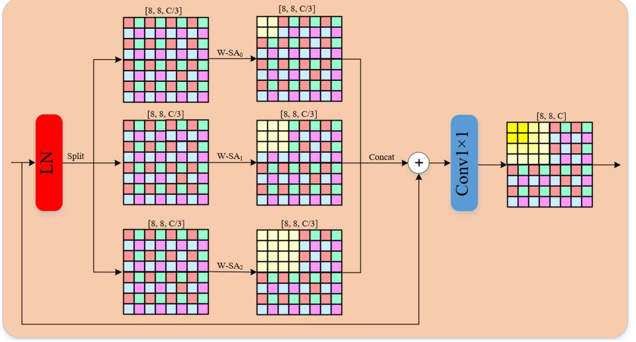
Fig. 6 Schematic of the window multi-scale self-attention.
