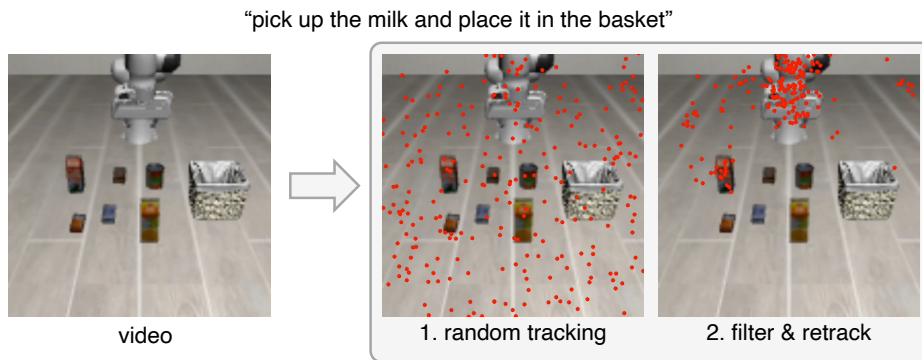
Figure 10. Given a video (left), we query 1000 randomly sampled points using an off-the-shelf TAP model (middle), where each colored dot represents the starting position of a track. We then filter the tracks using a heuristic of their position displacement across the video and re-sample about these points (right). From observation, the extracted tracks are concentrated around informative objects, such as robot’s gripper and manipulation targets.
