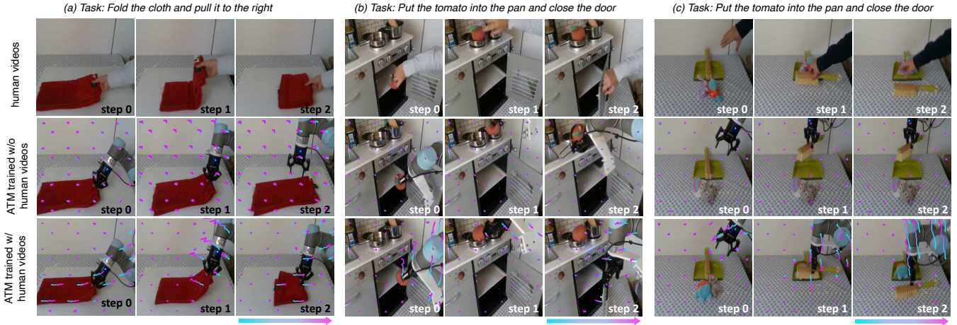
Fig. 6: Learning robotic skills from human videos for three tasks. We collect 100 videos of a human performing the tasks directly and 10 teleoperation demonstration trajectories. Each row from the top to the bottom shows three snapshots from the human videos, ATM trained without the human videos, and ATM trained with the human videos. By comparison, we can see that human videos are critical in learning accurate trajectory prediction and enable the policy to successfully perform the task.
