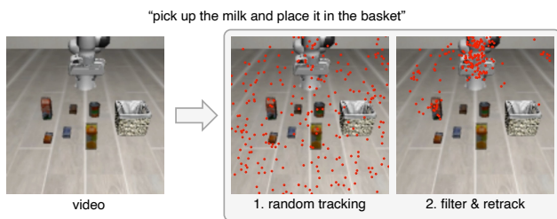
Fig. 12: Given a video (left), we query 1000 randomly sampled points using an off-the-shelf TAP model (middle), where each colored dot represents the starting position of a track. We then filter the tracks using a heuristic of their position displacement across the video and re-sample around these points (right). We can see that extracted tracks are concentrated around informative objects, such as the robot’s gripper and manipulation targets.
