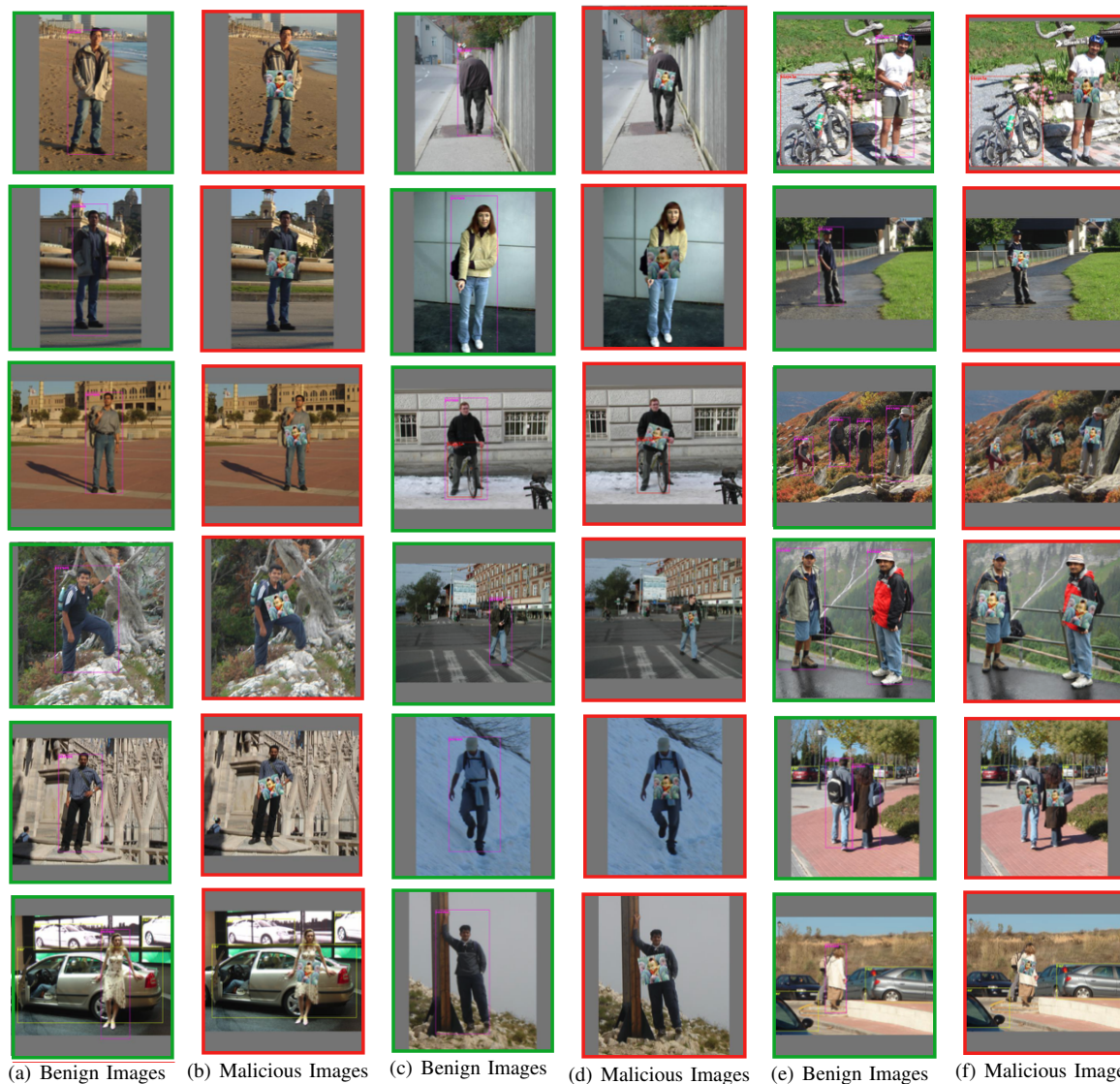
Fig. 7. Illustration of experimental consequence in the digital domain. The images with green rectangles represent the object detectors can recognize the class of a person successfully while the images with red rectangles denote the object detectors can not recognize the class of a person.
