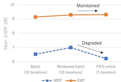
Fig. 9 Comparing MDP- and SWF-based scaling methods using TV Laplacian model; SWF-based scaling can prevent accuracy degradation between windowed batch and FIFO online algorithms and improve  $\Delta SDR$  scores for all algorithms.
