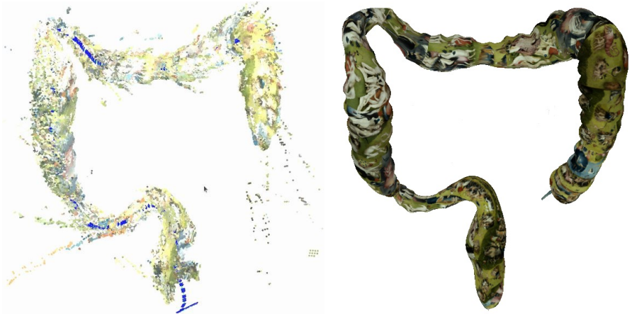
Fig. 4 3D reconstruction on the synthetic data set. Left is the full 3D recovered map of BDIS-SLAM. Right is the original 3D mesh for synthetic endoscopy data simulation.
