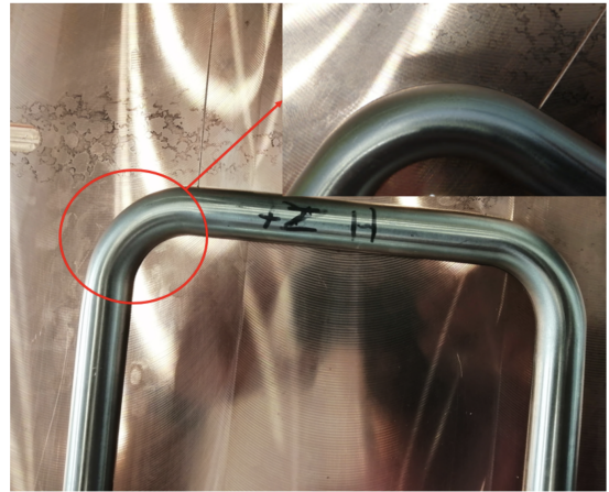
FIG. 13. Groove in CuCr1Zr plate machined with a 0.1-mm gap surrounding the tube’s bend region.
