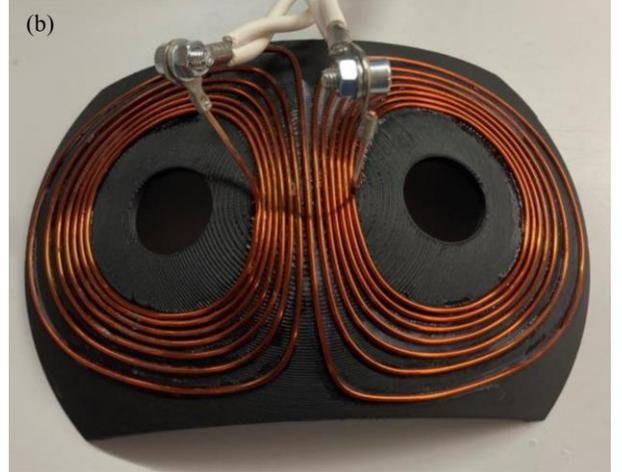
Fig. 3. Experimentally detected field and corresponding implementation of the coil from Fig. 2(b). (a) Plot of E-Field magnitude sampled under spherical constraints and (b) implemented experimental coil with 14 turns.
