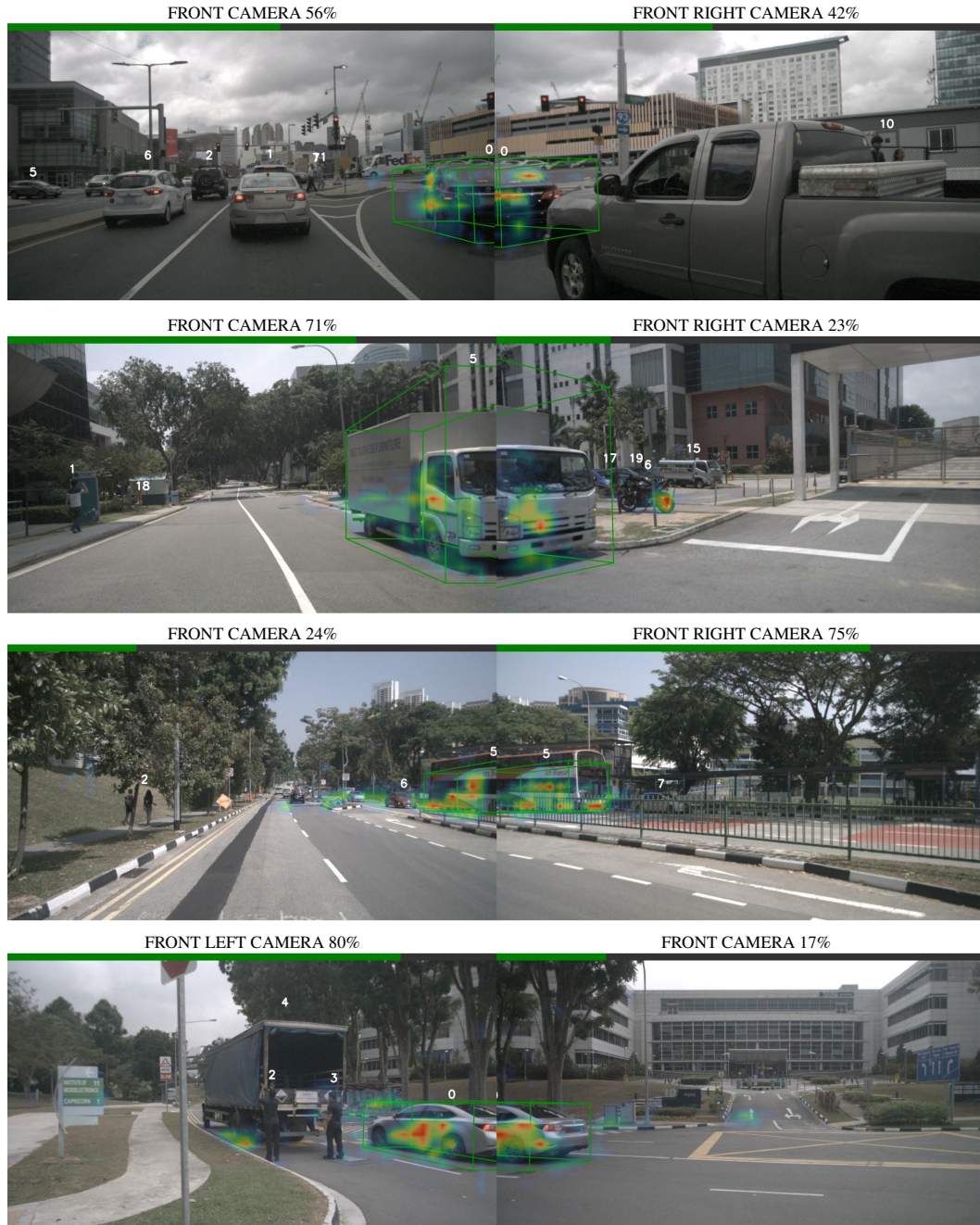
Figure 22: Raw cross-attention examples for objects (green OBB) that lie in the overlapping FOV of two cameras. In each example, a single query is used to generate the saliency maps for all camera images. Attention can be observed on the object on both overlapping camera images. We further approximated the contribution of each camera for a detection by computing the fraction of attention for each camera, indicated by the green bar and the percentage data.
