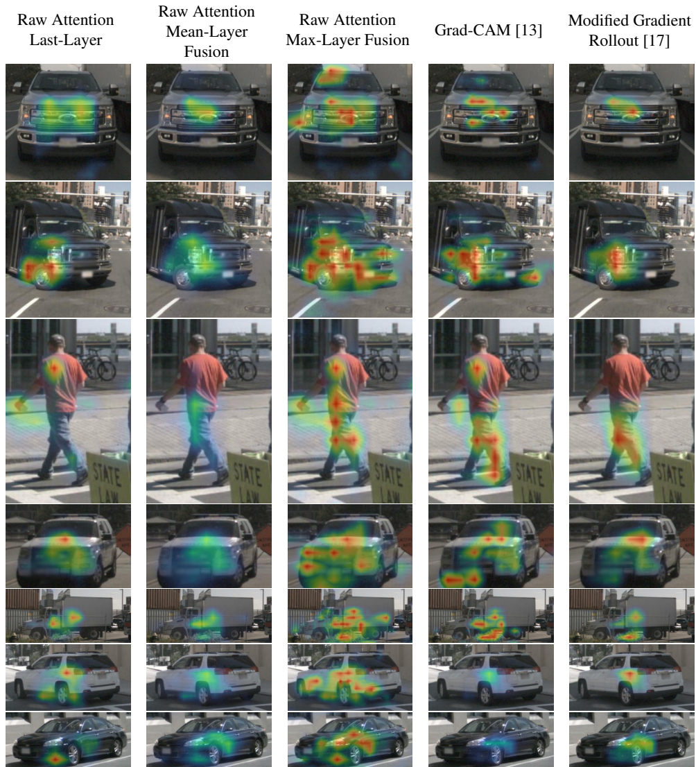
Figure 12: Saliency maps generated for Raw Attention (Last, Mean, Max), Grad-CAM and Gradient Rollout for different objects.
