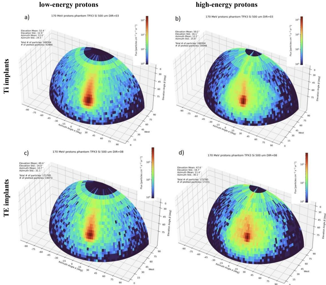
**Figure 6.** Directional maps of incident scattered protons selected from the data given in Fig. 3, for an angular position of  $60^\circ$  relative to the incident beam line. Results are given for data with the head phantom equipped with Ti implant (top row) and without (bottom row) the Ti implant (TE implants). The two selected spectral-tracking groups are shown: low-energy scattered protons (left column) and high-energy scattered protons (right column).
