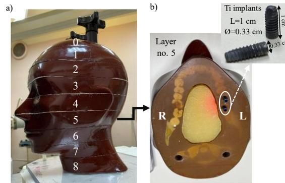
**Figure 1** *a) The anthropomorphic head phantom (Alderson phantom) made out from 9 independent layers that sum up the whole anatomy of the human head; b) two cylindrical metallic implants made from titanium (Ti) were inserted into the 5<sup>th</sup> layer of the Alderson phantom, at the molars' level.*
