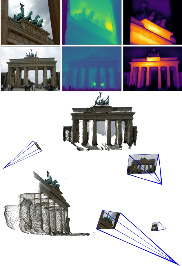
Figure 4. Example of 3D reconstruction of an unseen MegaDepth scene from two images (top-left). Note this is the raw output of the network, i.e. we show the output depthmaps (top-center, see Eq. (8)) and confidence maps (top-right), as well as two different viewpoints on the colored pointcloud (middle and bottom). Camera parameters are recovered from the raw pointmaps, see Sec. 3.3 in the main paper. DUS t 3R handles strong viewpoint and focal changes without apparent problems
