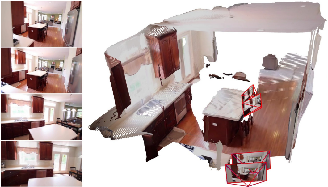
Figure 9. Reconstruction example from 4 random frames of a RealEstate10K indoor sequence, after global alignment. On the left-hand side, we show the 4 input frames, and on the right-hand side the resulting point-cloud and the recovered camera intrinsics and poses.
