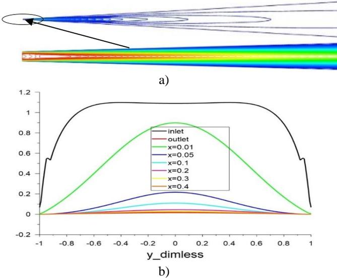
Fig. 4 The isolines of the averaged longitudinal component of the velocity  $\text{mean}_V_x$ , (below are the isolines of the  $\text{mean}_V_x$  velocity near the entrance to the diffuser) (a), the profiles of the longitudinal component of the  $\text{mean}_V_x$  velocity (b) for case  $V_{in} = 11.7$  m/s,  $A = 0.1$  m/s,  $f = 10$ Hz ( $Re=279$ ,  $Re_{vibr}=2.4$ )
