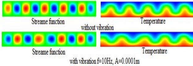
Fig. 6. Pictures of isolines of the stream function and isotherms with and without vibrations of the lower wall with  $Re_{vibr} = 0.007$ ,  $Ra = 4 \cdot 10^3$ ,  $Pr = 1$ .
