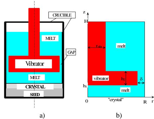
Fig. 8. The principal geometrical schemes for Bridgman crystal growth model with submerged vibrator, a) for Stefan problem with variable melt-crystal interface, b) model with fixed flat shape of the melt-crystal interface
