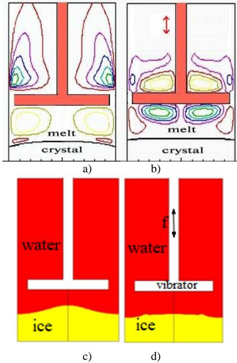
Fig. 10: The effect of vibrations on the shape of the front crystallization: a), b) – stream function in the melt of NaNO<sub>3</sub>, (a) without vibrations -  $f=0$ ; b) - with vibrations  $A=10^{-4}$  m,  $f=50$  Hz), c), d) – water-ice interface, c) – without vibrations,  $f=0$ , d) – with vibrations,  $A=10^{-4}$  m,  $f=30$  Hz)
