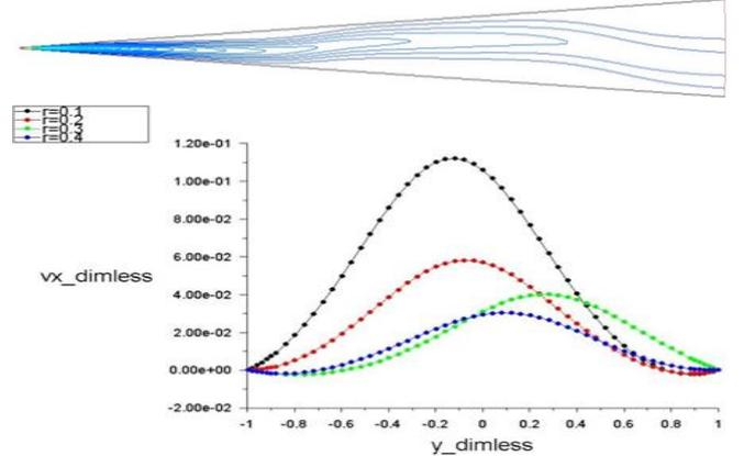
Fig. 2. The isolines and the profiles in vertical cross-sections of horizontal component  $V_x$  of velocity vector for the case of asymmetrical steady state fluid flows ( $Re = 279$ ).
