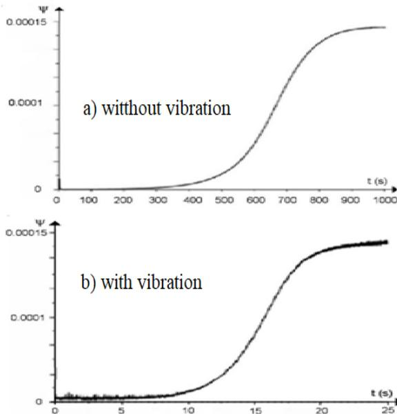
Fig. 7. The dependences of the maximum values of the stream function on time ( $Ra = 4 \cdot 10^3$ ,  $Pr = 1$ ): a) – without vibrations; b) – with vertical vibrations of the bottom wall with  $Re_{vibr} = 0.007$ .
