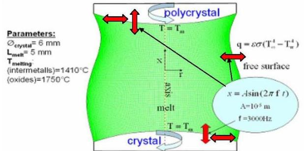
Fig. 13. The scheme calculation region for floating zone model
