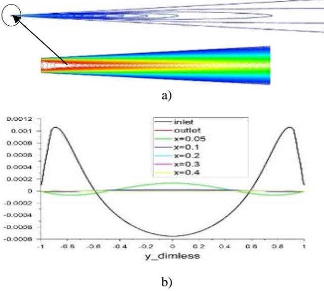
Fig. 3. The isolines of the averaged longitudinal component of the velocity  $\text{mean}_V_x$ , (below are the isolines of the  $\text{mean}_V_x$  velocity near the entrance to the diffuser) (a), the profiles of the longitudinal component  $\text{mean}_V_x$  of the velocity (b) for case  $V_{in} = 0$ ,  $A = 1$  m/s,  $f = 10$  Hz
