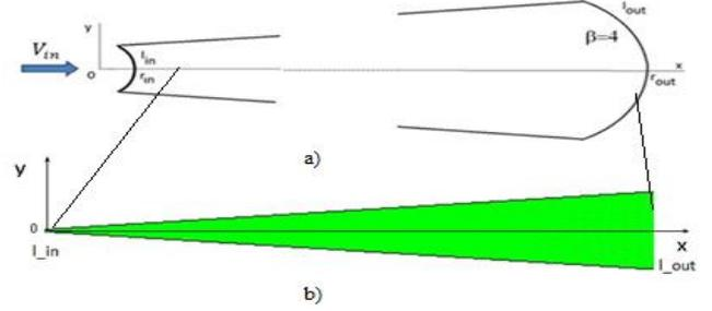
Fig. 1. Scheme of the computational domain for a flat diffuser: a) it is details of domain near the inlet and outlet of the diffuser; b) the numerical region with mesh ( $\beta = 4^\circ, L = 0.495$  m).
