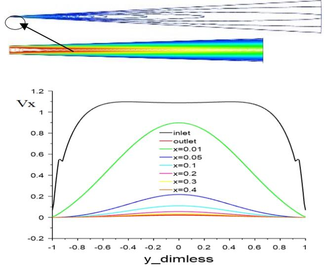
Fig. 5. The profiles of time average velocity ( $\text{mean}_V_x$ ) for fluid flow in a flat diffuser with vibration action from the walls of the diffuser for  $Re=279$ ,  $A=0.001$ m/s,  $f=10$ Hz ( $Re_{vibr}=0.02$ ).
