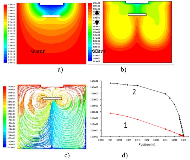
Fig. 12. Isotherms temperature: a) – without vibration, b) with vibrations c) flow tracks, d) temperature profiles on the axis section: curve 1 - is without vibration, curve 2 - is with vibration. ( $Pr=7$ ,  $Re_{vibr} = 1500$ ,  $Ra=0$ ).
