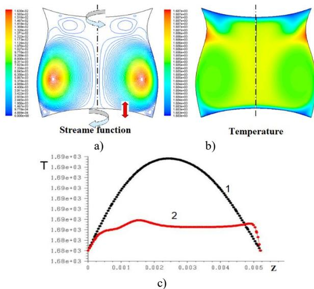
Fig. 14. a) – Stream function, b)- Isotherms in the melt Si ( $Pr=0.01$ ) with natural and Marangoni convection, rotation, and vibrations. c) - vertical temperature profiles ( $r=0.75$ ) (line 1 – without vibrations, 2 – with vibrations bottom wall ( $A=10^{-4}$  m,  $f=3\text{kHz}$ )).
