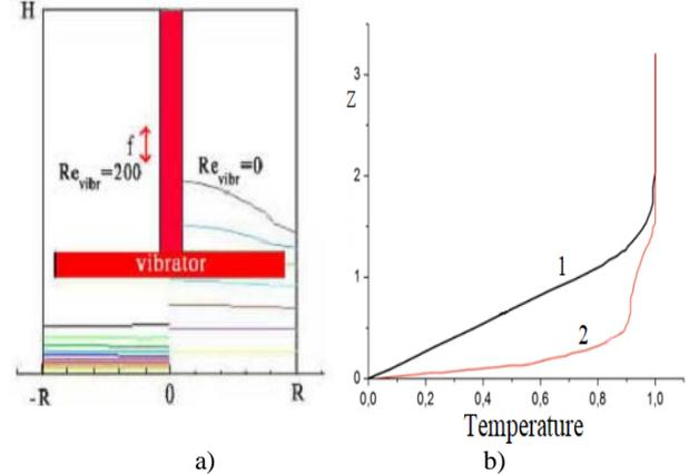
Fig. 9. a) - Isotherms in the  $NaNO_3$  melt ( $Pr=5.43$ ) (on the right – without vibrations, on the left – with vibrations  $Re_{vibr}=200$ ), b) - vertical temperature profiles ( $r=0.75$ ) in the  $NaNO_3$  melt ( $Pr=5.43$ ) (line 1 – without vibrations, 2 – with vibrations  $Re_{vibr}=200$ )
