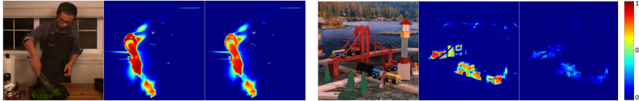
Fig. 3: Dynamic MLPs with tunable parameters \alpha weigh the parameters of the MLP for each Gaussian. We show renders from two scenes, left: cook spinach [25] and right: Train [51]. Shown from left-to-right: image render, tunable \alpha parameters, and normalized MLP displacements \Delta\mathbf{x} . Note, \alpha highlights the scene’s dynamic regions.
