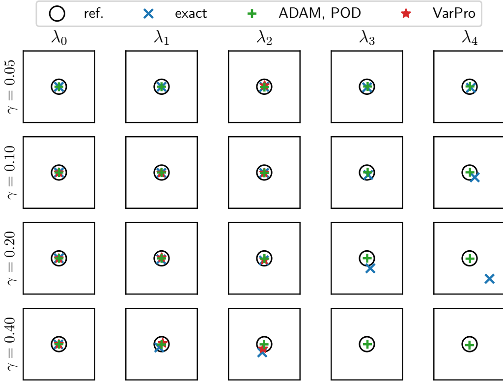
Figure 5: Cylinder flow example: comparison of the five most dominant eigenvalues (sorted by amplitude) for different noise levels \gamma . The truncation rank is r = 20 . The exact DMD applied to the clean data is used as a reference. For clarity, we have omitted the ADAM markers because the results were nearly identical to ADAM/POD. Each subfigure has a width and height of 0.01.
