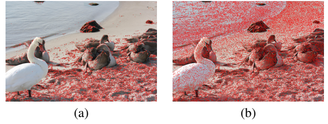
Fig. 1. Keypoint detection by (a) classical contrast threshold; (b) reducing contrast threshold.
