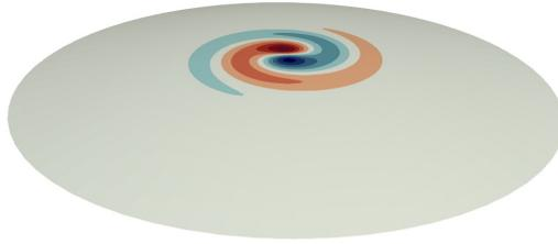
Figure S2: Eigenmode of the temperature field of the azimuthal thermal Marangoni instability ( $m = 1$ ) of a non-volatile droplet on a heated substrate, which perfectly agrees with Fig. 12(a) of Ref. [31]. In their work, they obtained a critical Marangoni number of 122.0, our bifurcation tracking yields 121.96. This indicates that the explicit treatment of the viscous term for  $m = 1$  seems to be redundant.
