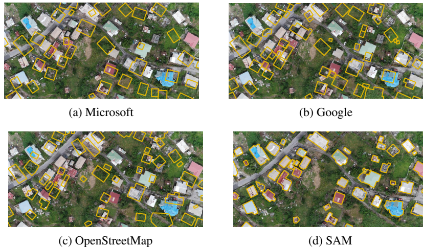
Figure 2: Building footprints from (a) Microsoft, (b) Google, (c) OpenStreetMap, and (d) SAM overlaid on a drone image taken in Salisbury, Dominica from OpenAerialMap [5].
