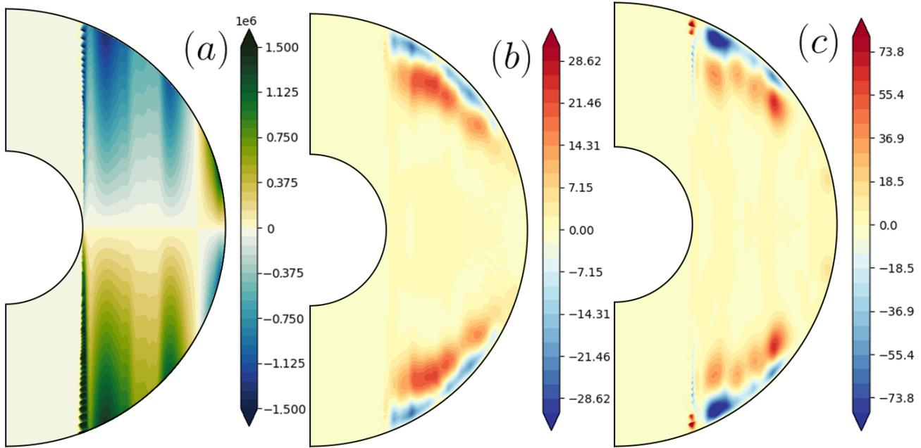
**Figure 4.** (a) Meridional section of the longitudinally-averaged 3D-helicity  $\overline{\mathbf{u}_{3D} \cdot \nabla \times \mathbf{u}_{3D}}$ . (b) Azimuthal component of the mean electromotive force  $\overline{(\mathbf{u}'_{3D} \times \mathbf{B}') \cdot \mathbf{e}_\phi}$ . (c) Estimated mean  $\alpha$ -effect  $-\frac{d}{3\{\mathbf{u}'_{3D}\}_S} B_\phi \cdot (\mathbf{u}'_{3D} \cdot \nabla \times \mathbf{u}'_{3D})$ . For the same case as in Fig. 3.
