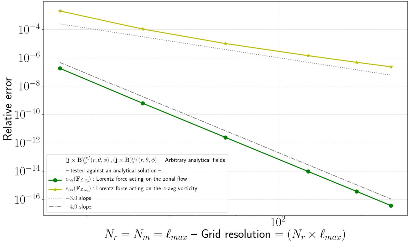
**Figure A1.** Convergence of the relative error of the Lorentz force terms tested against an analytical solution.
