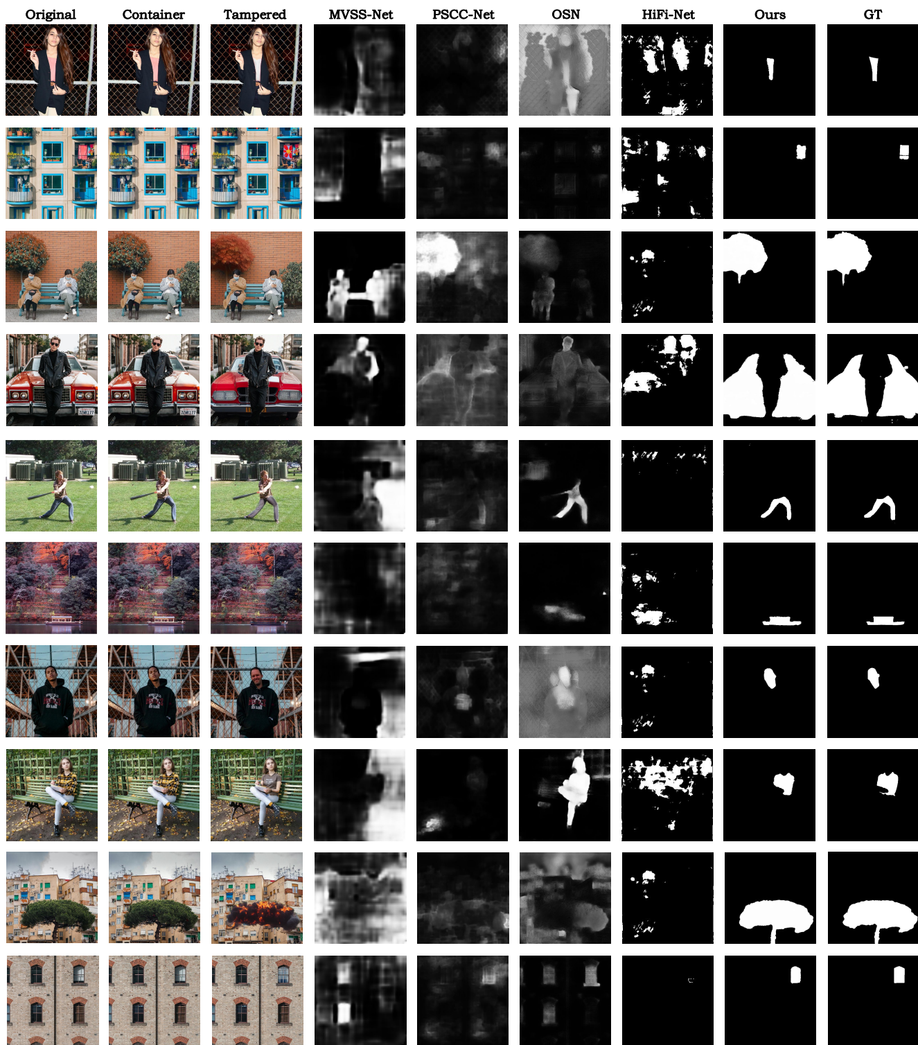
Figure 15. Localization results of our EditGuard and other methods [12, 23, 46, 78] on the constructed AGE-Set-F. The tampered images are manipulated by AIGC-based editing software with some customized models and well-designed prompts, and are hard for the naked eye to detect. In these cases, almost all methods fail but our EditGuard can still precisely produce the tampered masks. Zoom in for a better view.
