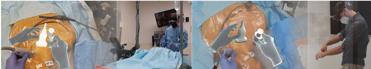
Figure 1: Mixed reality communication for medical procedures. We present a mixed reality communication system. A remote expert (right) guides a local operator (left) through the placement of a central venous catheter using augmented objects.
