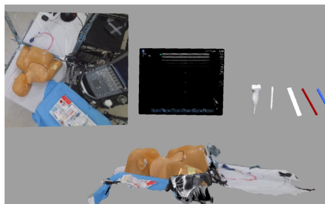
Figure 4: Remote view. The remote virtual workspace consists of the volumetric view (bottom center), the video feed (left), the ultrasound feed (top center), and the virtual objects (right). The virtual workspace can be placed in any room.
